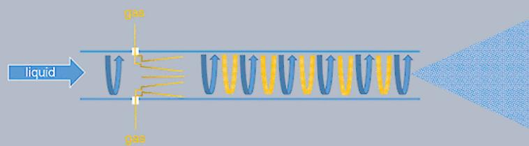
**front view turbiti static mixer with swirl flow technology**
